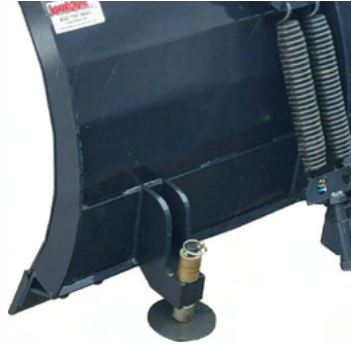
Adjustable Skid Shoes — to ensure that you're not taking off sod or grave; during snow clearing
