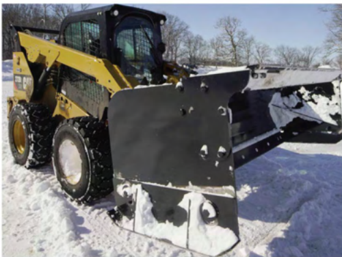
Side Plates Full trip edge and free floating side plates
