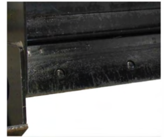
Cutting Edge Heavy-duty 3/4" thick
